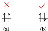
**Figure 2.1** According to Pauli's exclusion principle, the situation as showed in figure (a), where two electrons of the same spin occupies the same quantum state is not allowed. Whereas, as shown in (b), two electrons of opposite spin are allowed to occupy the same quantum state.
